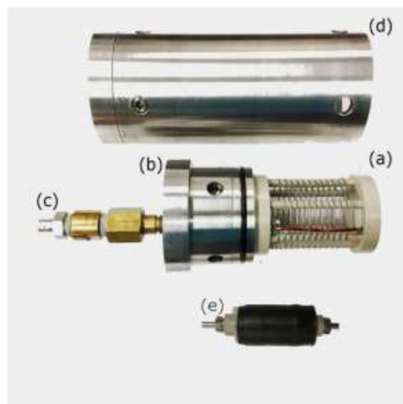
FIG.1. The experimental core holder: (a) open frame RF probe, (b) Hastelloy-C metal end cap closure, (c) high pressure BNC connector, (d) MR/MRI compatible metal core holder, including the vessel and the end cap, (e) Berea sample was enclosed by fluid distributors, sleeve and heat shrink tubing. The enclosed sample was placed inside the open frame RF probe during high pressure MR/MRI measurements.
